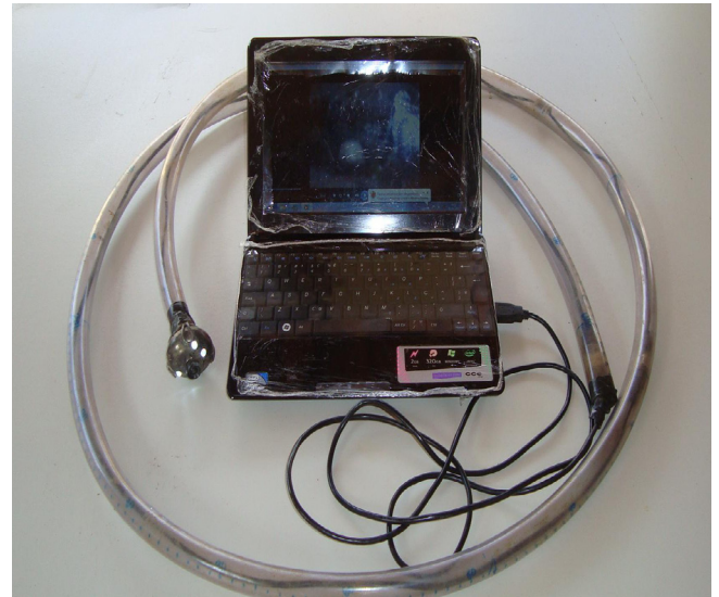
FIGURE 1. Probe attached to a netbook used to visualize the Momotus momota nestlings.
